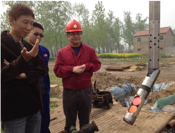
DSC 测井仪器下井
